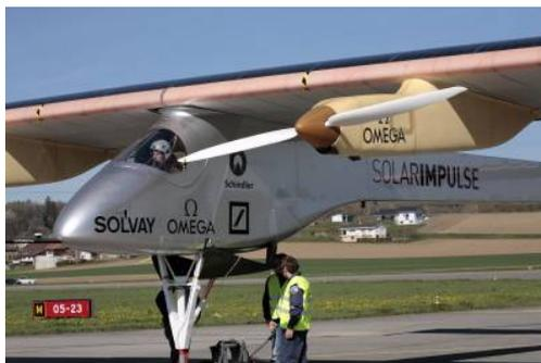
**Ixef® polyarylamide (PARA)** is used in the landing gear mechanism of Solar Impulse.
