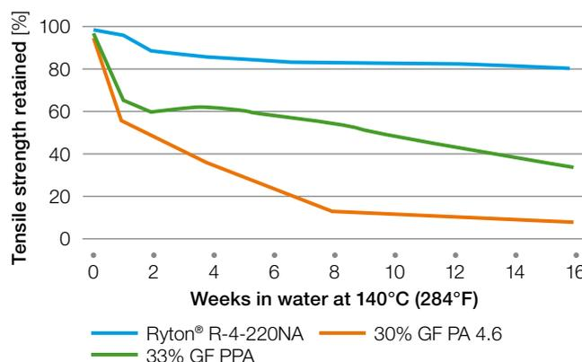
Immersion tests have also shown Ryton® PPS to be essentially unaffected by low concentrations of
