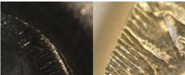
**Figure 8:** Pattern representative of severe chemical attack in sulfone polymers
