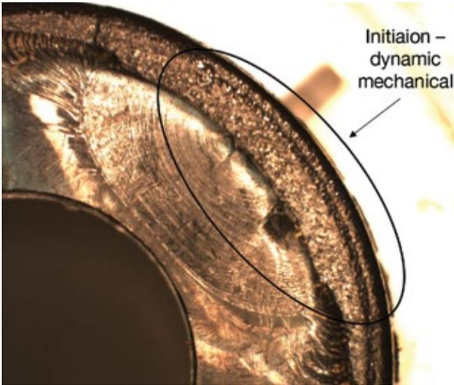
**Figure 6b:** Coexistence of two different failure processes, which switches from original dynamic mechanical failure into a rapid propagation (static mechanical failure)
