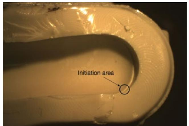
**Figure 6a:** Coexistence of two different failure processes, which switches from original dynamic mechanical failure into a rapid propagation (static mechanical failure)
