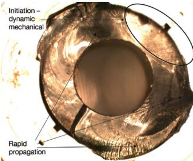
**Figure 7:** Pattern representative of moderate chemical attack in sulfone polymers
