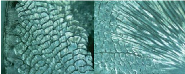
**Figure 4:** Crocodile-skin pattern subsequent to a mechanical failure as the propagation rate increased
