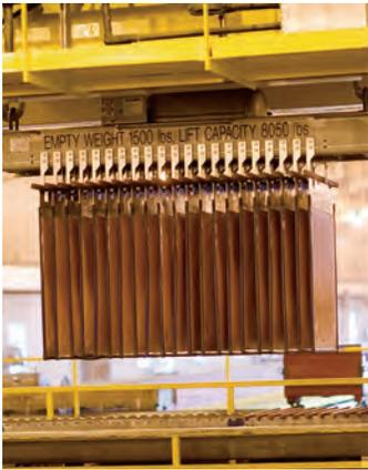
Copper cathode is being harvested in the tank house at a Cytec customer site that uses our ACORGA® reagents to purify and concentrate the copper.
