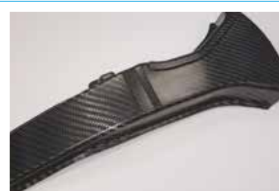
B Pillar manufactured from SolvaLite™ 730
