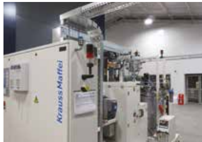
HP-RTM equipment in Application Center
