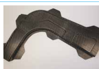
A Pillar manufactured from SolvaLite™ 730
