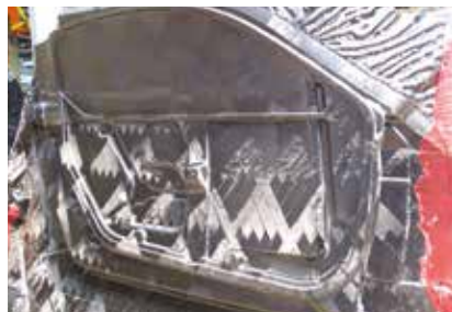
Door inner frame after pressing
