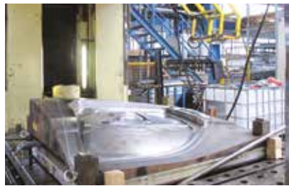
Stamping of the blank in a two-sided metal mold using a hydraulic press
