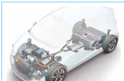
Chevrolet Spark EV battery tray manufactured from SolvaLite™ 23
