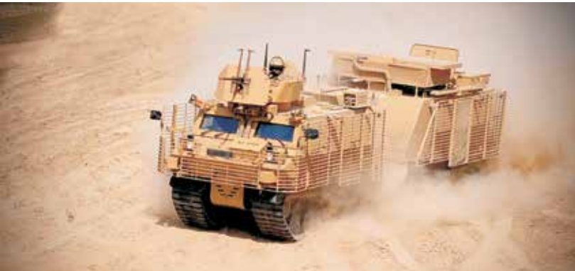
Appliqué armor and spall liners applications on the UK MoD's Warthog vehicle.
