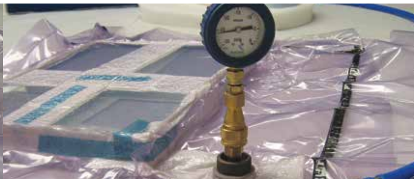
Figure 11. Shows the vacuum gauge and socket assembly attached to the vacuum breach unit.
