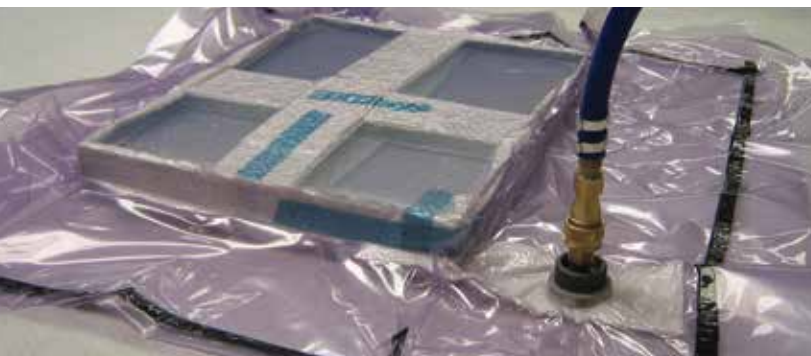
Figure 10. The vacuum hose and socket unit are attached to the vacuum breach unit, allowing air to be evacuated and vacuum applied. If the position of the bag needs adjusting (i.e. if bridged), the hose can be easily and quickly disconnected. To release vacuum depress the nipple of the non-return plug and manipulate the film as required.
