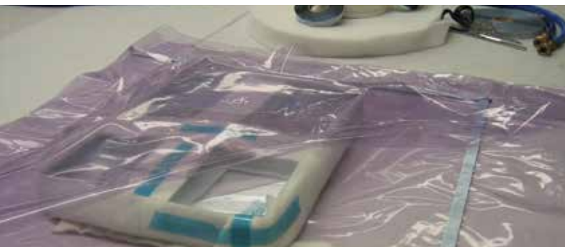
Figure 3. Sealant tape attached to the vacuum film. Release paper should be left in place until ready to complete the bagging process. Note that the lower part of the vacuum breach unit must be positioned prior to sealing the bag together.
