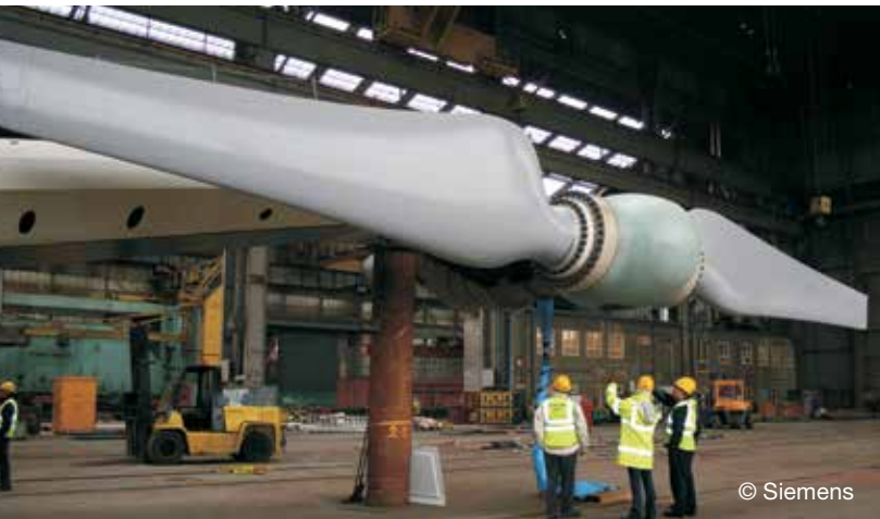
SeaGen composite blades, manufactured by Aviation Enterprises Ltd, made from Solvay's VTM® 260 series prepregs
