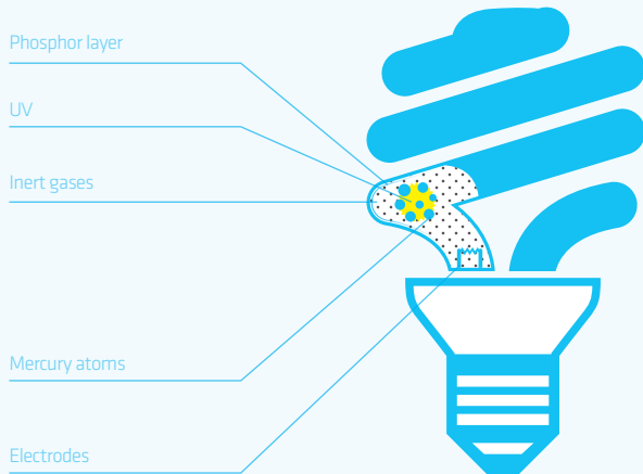
Structure of an energy saving lamp
