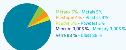
Exemple de composition de poudre de luminophores - Example of composition of phosphor powder
