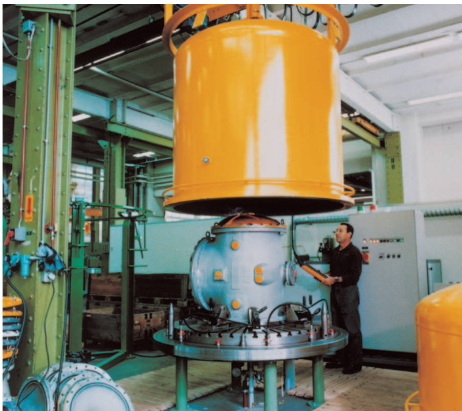
Fig. 38 Leak testing of a GIS aluminium housing (ABB, Switzerland)
