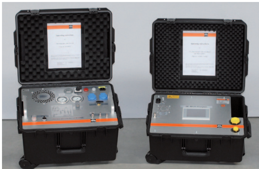
Fig. 41 SF 6 measuring devices (DILO, Germany)
