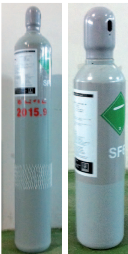
Fig. 47 and Fig 48 SF 6 -cylinders 47 l and 10 l from Onsan plant
