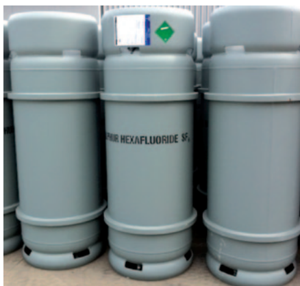
Fig. 49 SF 6 -pressure drums 600 l from Onsan plant
