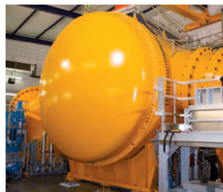
Fig. 20 300 kW electron processing system consisting of two 3 MeV accelerators (Vivirad, France)
