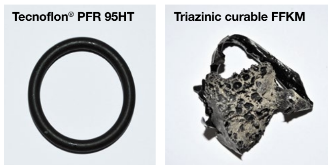
Effect of steam: 1 week @ 300^{\circ}\text{C}
