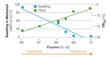
Tecnoflon® FKM bisphenol curable grades are copolymers and terpolymers with a fluorine content range from 66% to 70% and are well suited for:
