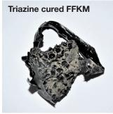
Thanks to its specific proprietary cross-linking chemistry, Tecnoflon® PFR 95HT shows negligible physical properties loss after 1 week at 300°C steam exposure, largely outperforming triazine cured FFKMs that are severely degraded in the same conditions (see the pictures on the left).
