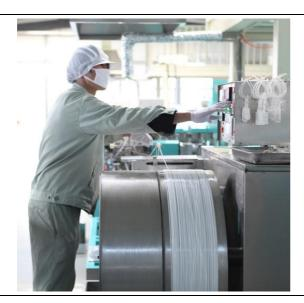
Scinor Beijing Membrane Technology chose Solvay's Solef® PVDF to optimize its thermally induced phase separation (TIPS) membrane technology, which has applications in reverse osmosis pretreatment as well as industrial and drinking water applications. Solef® PVDF's narrow molecular weight distribution and more uniform bulk density enabled Scinor to achieve more stable extrusions that help optimize the performance and reliability of its TIPS membranes. Photo courtesy of Scinor.
