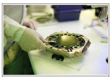
Solvay's new <u>Halar® ECTFE</u> waterborne coating system enabled Southwest Impreglon (SWI), a specialty coatings company, to coat silicon wafer processing equipment with highly complex geometries. Halar® ECTFE waterborne coating system allows for a smooth, uniform, pinhole-free surface for high-quality corrosion protection on intricate parts that are not suitable for electrostatic powder coating. Photo courtesy of Solvay.
