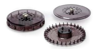
Radel<sup>®</sup> PPSU resin's high transparency, superior chemical resistance, ability to withstand repeated steam sterilization and compatibility with ultrasonic welding led ELITechGroup Biomedical Systems to choose it over other transparent thermoplastics to upgrade two injection-molded carousels used in ELITechGroup's industry-leading diagnostic slide staining tools. Photo courtesy Solvay Specialty Polymers.
