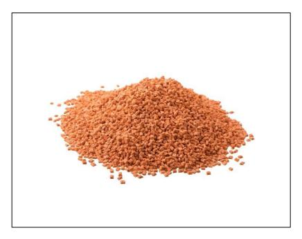
Ixef® 1524 RD 001 is a halogen-free flame retardant (HFFR) and 50 percent glass fiber reinforced polyarylamide (PARA) grade color matched to signal orange, for high-performance electrical vehicle (EV) recharge connectors. Photo: Solvay
