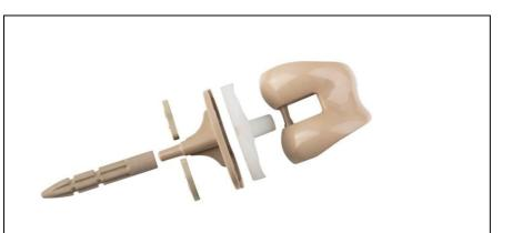
Okani Medical Technology, a China-based pioneer in artificial joint applications, developed its ORGKnee™ all-polymer knee implant, based on Solvay's Zeniva® polyetheretherketone (PEEK). Test simulations of the implant indicate that PEEK helped reduce wear by 50 percent versus a metal implant as measured by material loss over 3 million cycles. Photo courtesy of Okani Medical Technology.
