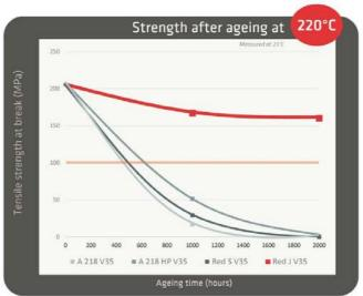
Tensile strength after ageing: Test results have confirmed that 2,000 hours of working temperature at 220°C are perfectly manageable with Solvay's cost-effective new Technyl® Red J high-heat technology for automotive turbo engine components. Graphic courtesy Solvay Performance Polyamides.
