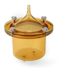
Solvay's tough, transparent, biocompatible Radel® R-5000 polyphenylsulfone replaced polyetherimide as Biorep Technologies' material of choice for its new Ricordi chamber, used to isolate healthy pancreatic tissue cells for clinical transplants. Photo courtesy of Solvay Specialty Polymers.
