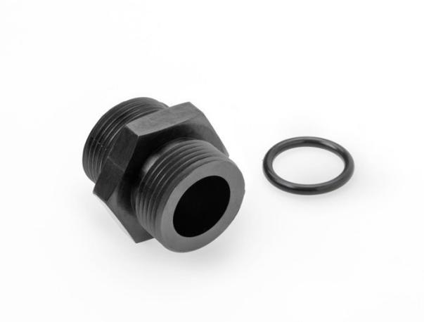
The Polimotor 2 project chose Solvay Specialty Polymer's Amodel® A-8930 HS polyphthalamide (PPA) to fabricate the water inlet/outlet fixture in its advanced race engine. Solvay's high-performing reinforced grade of PPA withstands high temperature automotive coolants better than polyamide 66. It also expands design options for automotive cooling system components as automakers contend with rising underhood temperatures. Photo courtesy of Solvay Specialty Polymers.
