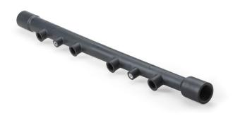
Above: The Polimotor 2 all-plastic engine project selected Solvay's Ryton® XK2340 polyphenylene sulfide (PPS) reinforced resin to injection mold its engine's 46-cm (18-in) fuel rail component. Replacing the typically steel part with a high performance thermoplastic not only allowed the fuel rail to be injection molded as a single piece, it also enabled 25 to 30 percent reduction in part weight.
