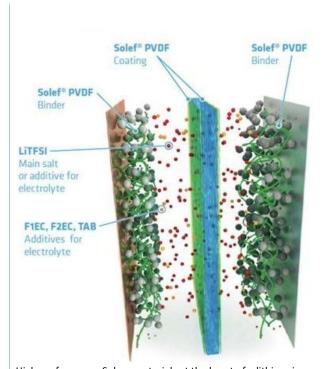
High-performance Solvay materials at the heart of a lithium-ion battery: The PVDF separator coating helps to maintain the lamination among separator and electrodes even at high temperature, while binders ensure the electrode integrity during cycling. Advanced electrolyte additives enhance the life, capacity and safety of the cell.
