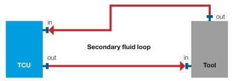
The products offered for use in heat transfer applications are called Galden<sup>®</sup> HT. This is a line of dielectric fluids with boiling points ranging from 55 °C to 270 °C. Galden<sup>®</sup> PFPE excellent dielectric properties, high chemical stability combined with their capacity to operate at very low as well as elevated temperatures make them the best heat transfer fluids for the aggressive conditions found in many semiconductor processes, electronic, and solar industries.
