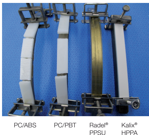
Figure 2: Test bars after 7-day exposure to Virex® TB under high constant bending stress (30 MPa)
