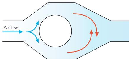
Back side of a round tube has low heat transfer, causes pressure drag, and is a source of noise.
