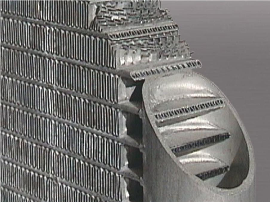
Brazed heat exchangers also offer a higher mechanical resistance, especially in the fin connection, so that even incorrect handling or accidental collisions cause less deterioration with time.
