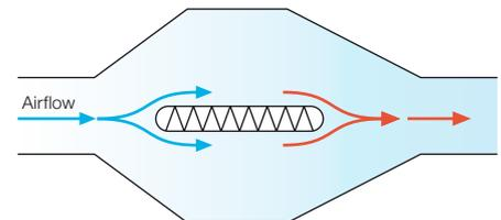
Back side of flat tube has improved heat transfer, reduced pressure drop with lower noise.
