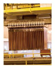
Copper cathode is being harvested in the tank house at a Cytec customer site that uses our ACORGA® reagents to purify and concentrate the copper.
