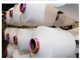
Solvay has developed a new polyamide fiber which "deactivates" viruses such as Covid-19 and eliminates bacteria. The permanent anti-bacterial additive used in the composition of the fiber prevents the transmission of bacteria and therefore reduces the risk of contamination. This fiber could be used for car or airplane seats, or any application where people could be in contact with textiles that cannot be washed or disinfected daily.
