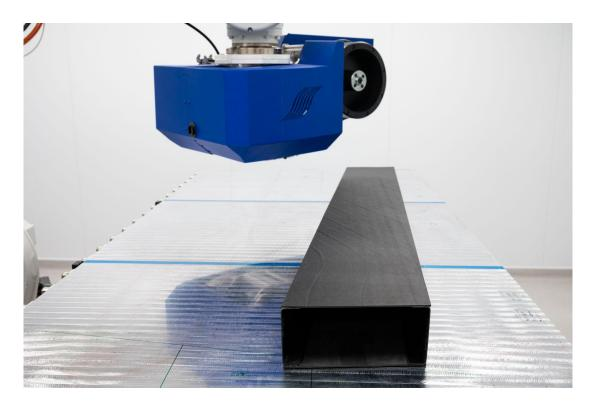
Wingbox demonstrator manufactured using iCOMAT's Rapid Tape Shearing (RTS) process and Solvay's CYCOM<sup>®</sup> EP2190 unidirectional prepreg.
