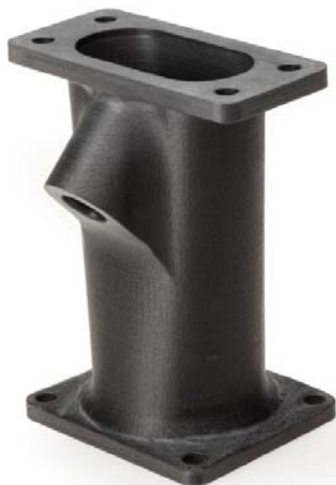
Fuel intake runner for the Polimotor 2 all-plastic engine, 3D printed in a reinforced Filament Fusion process using 10 percent glass filled KetaSpire ® PEEK polymer. (Photo courtesy of Solvay)
