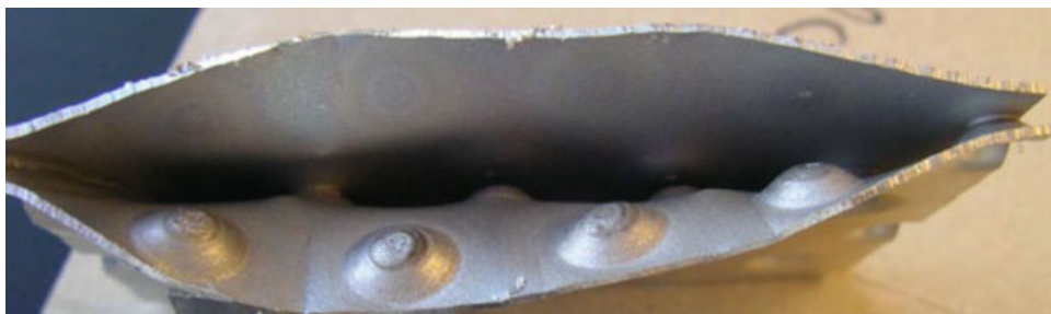
Figure 11. Not-brazed dimples. Plate mechanically opened up after the brazing
